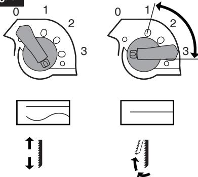
**⚠ WARNING** To reduce the risk of injury, always allow the jig saw to come to a complete stop before changing the orbital function setting.
