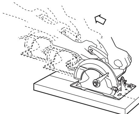
**Do not use dull or damaged blades.** Unsharpened or improperly set blades produce narrow kerf causing excessive friction, blade binding and kickback.
