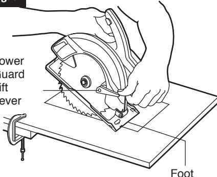
**WARNING** Once the foot plate rests flat on the surface being cut, release the lower guard and move the hand holding the front of the foot plate to hold the auxiliary handle. Proceed cutting in forward direction to end of cut.
