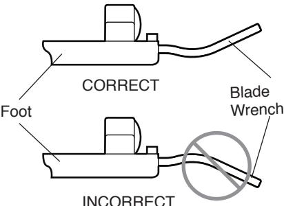
Wrench storage is provided on the tool (Fig. 3). Wrench is fully seated when second lock detent is engaged.
