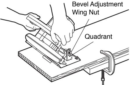
Disconnect plug from power source. The foot can be adjusted up to 45° by loosening the bevel adjustment wing nut at the front of the saw. Align to desired angle on calibrated quadrant. Then tighten bevel adjustment wing nut (Fig. 6).
